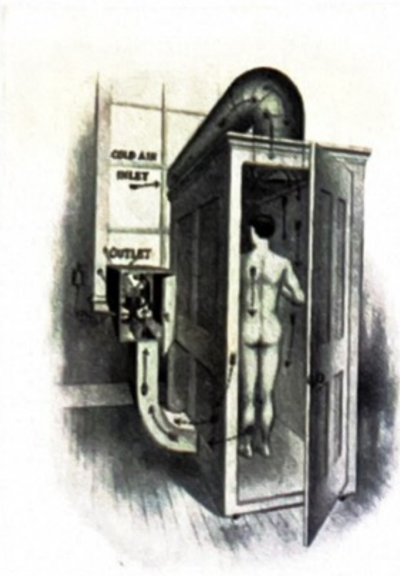
Fig. 14. Cabinet method of cooling the surface of the body with Electric Fan. See page 70.
